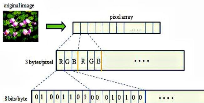
Figure 1. Accessing the Bits of a PNG image.
